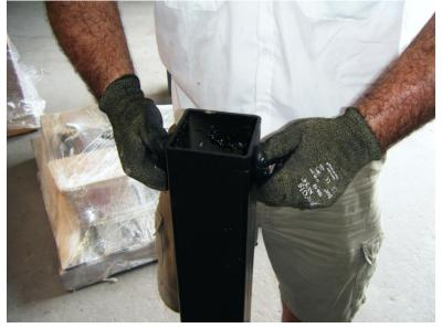
8. Once the two halves are separated you should see the inner screw with a bearing set on top. Rotate the inner tube to a position that the pull pin is at the desired direction.
