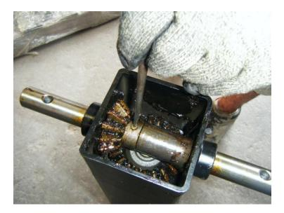
4. Remove the pin and set to the side. Slowly pull the cross shaft out of the jack removing the gear and the spacer shaft. Make reference to which side the gear is located on the cross shaft and the order of the parts.
