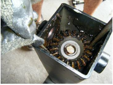
6. Under the gear you will find a second roll pin which supports the weight of the bottom leg. Insure the bottom leg of the jack is supported and the pin should easily slide out of the jack.
