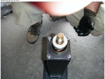
9. Re-assemble jack in reverse order. Insert inner leg and re-install the lower pin, replace the lower miter gear, install gear set and spacer on cross shaft. Re-install the pin into the upper gear and shaft. Test jack to insure smooth operation and grease. Re-install cap and two screws and you are complete.
