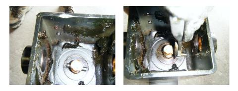
7. Once the bottom roll pin is removed the inner leg is ready to be separated from the outer leg. With the inner leg on a flat surface raise the upper tube off of the inner leg. Note: they should slide apart easily.
