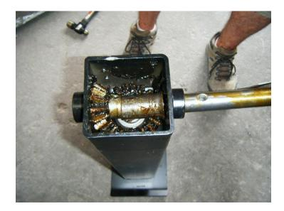
5. After removing the cross shaft, top miter gear, and spacer you should see the lower miter gear. With lower miter gear exposed raise lower miter gear straight up. Note: nothing is holding in the lower miter gear except the upper miter gear and cross shaft.
