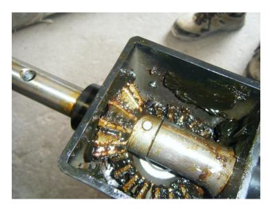
3. Drive the gear retaining pin out of the cross shaft. Note: start removing the pin and rotate the shaft so the pin is removed at an angle so it does not jam against the bottom gear.
