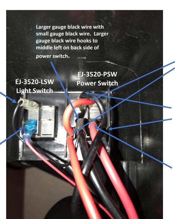
Large gauge red wire with additional large gauge red wire. Dual portion hooks on lower left on back side of power switch. Shorter section of large gauge red wire hooks on upper right on power switch.
