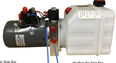
Hydraulic line for port A on HPU unit to run to port P on diverter. (Maximum pressure 3200 psi)
