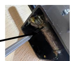
You will then be able to slide out the handle/gear shaft assembly.
