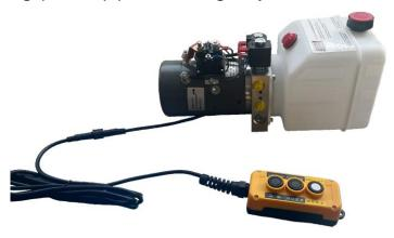
HPU-DAGDMD004 Dual acting, power up/power down/gravity down/manual down, 3-button switch, 4 quart reservoir
