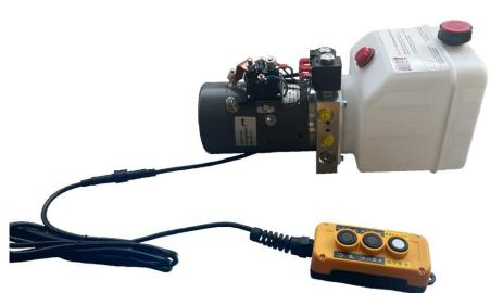
Hydraulic power units and control switch/remote pendant works with *RAM* hydraulic jacks and scissor hoist systems. •Works with 12 volt deep cycle direct current RV/Marine trailer battery (not supplied) •1.6KW 12v DC motor •Dual acting – Power Up/Power Down/Gravity
