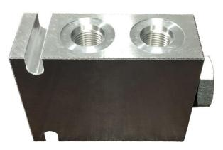
Use when operating two hydraulic jacks with one HPU •Receives flow from port A on HPU then divides the flow equally to run two hydraulic jacks •All ports are SAE #6 O-Ring female, requires adapters to couple with 9/16-18 SAE #6 JIC 37 degree flare hydraulic hose •HFD-612 Flow Divider
