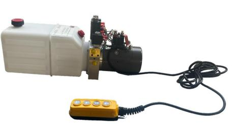
Hydraulic power units and control switch/remote pendant works with *RAM* hydraulic jacks and scissor hoist systems. •Works with 12 volt deep cycle direct current RV/Marine trailer battery (not supplied) •1.6KW 12v DC motor •Dual acting – Power Up/Power Down •3200 psi extension and 1500 psi retraction working pressure •2 to 4 selector allows use with bydraulic iack(s) and
