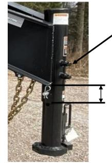
Set bolts are to face front of trailer toward tow vehicle. Set bolts are to torqued at 90 ft lbs.
