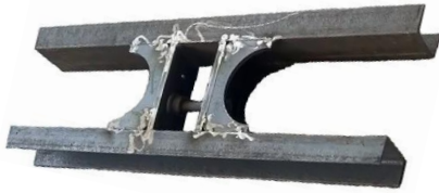
H bracket base to attached to the trailer frame
