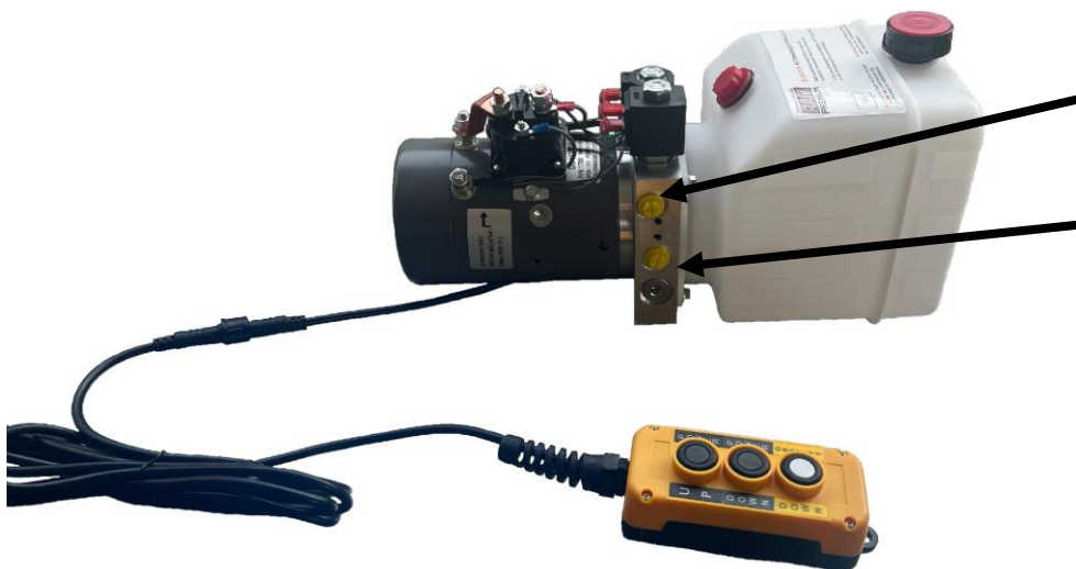
Port A – Extend / Fluid flow out of HPU
