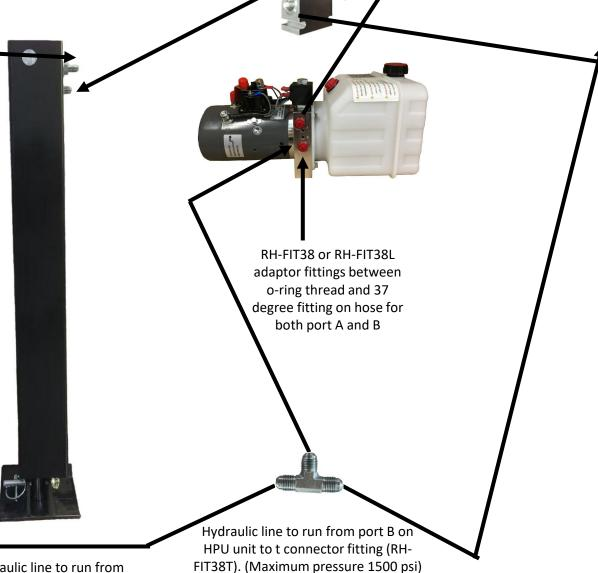
Hydraulic line to run from retract port (upper one) on jack to t connector fitting. (Maximum pressure 1500 psi)
