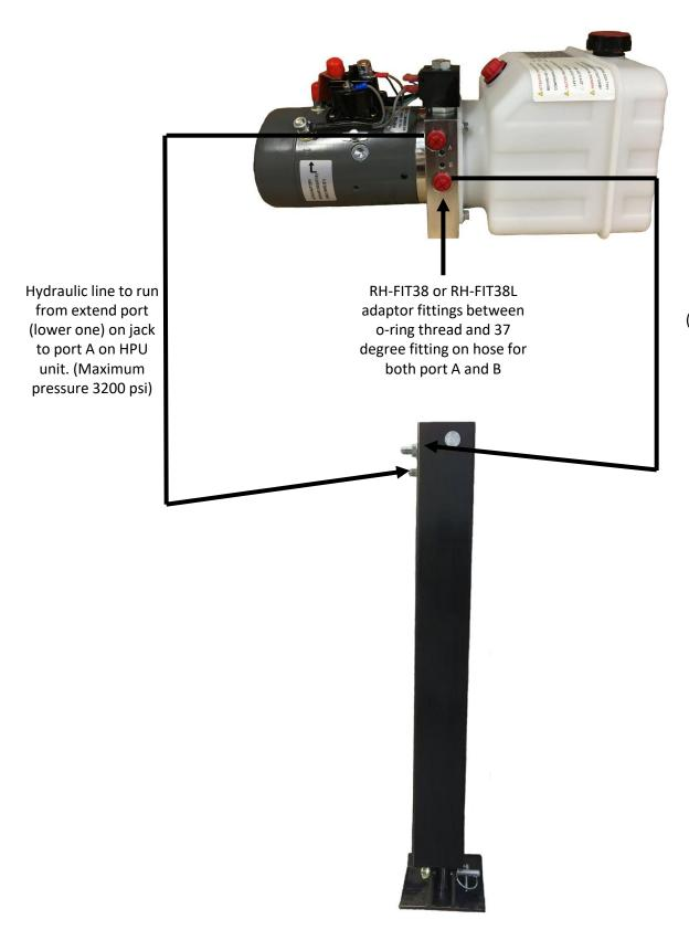
Hydraulic line to run from retract port (upper one) on jack to port B on HPU unit. (Maximum pressure 1500 psi)
