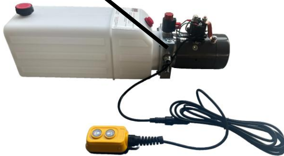
HPU is set up to receive 9/16-18 SAE #6 JIC 37 degree flare fittings. Cylinder is setup to receive SAE #8 ORB
